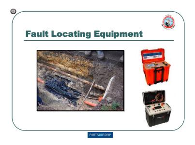
Various types of cable fault-locating equipment are available. When correctly used, ground fault locator and cable fault locator equipment can accurately identify the location and depth of underground cable, even when it is inside conduit, and can pinpoint breaks or faults in underground cable.
