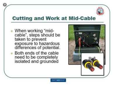
When working "mid-cable", steps should be taken to prevent exposure to hazardous differences of potential. Isolation requires both ends of the cable to be completely isolated.
