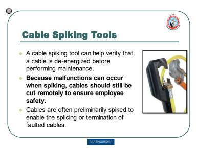
**Note:** Remote cable cutters and the cable spiking tool typically have written operating and safety instructions that must be strictly followed when operating these devices.
